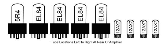
**RECTIFIER TUBE:** 5R4/GZ34. Replace only with high quality 5R4/GZ34 (or compatible) tube.
